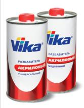
Acrylic thinner 1301-M (sluggish) is recommended for the painting of large areas as well as for elevated temperature conditions. It provides slower drying of a coating to a dust-free state, lessens overspray while applying the second layer.
